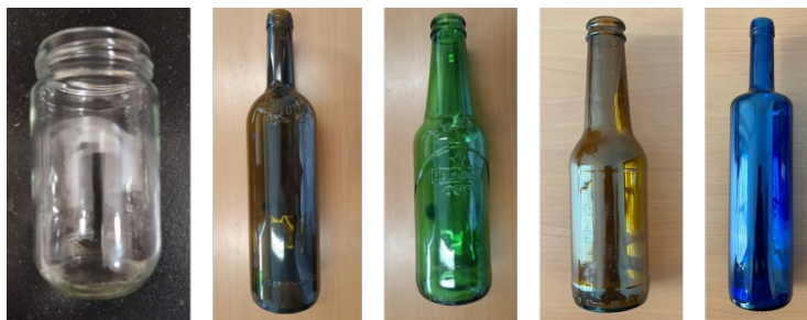
Figure 7 Picture of the containers, from left to right: white container, wine bottle (green), beer bottle (green and amber), and water bottle (blue).
